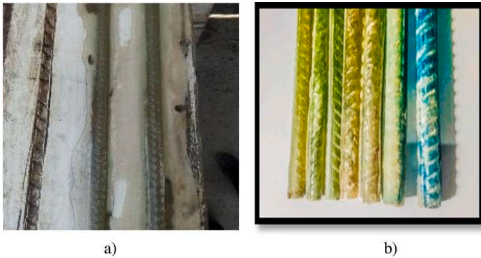
Fig. 1. GFRP bars; a) GFRP bars Manufacturing, b) GFRP bars diameters.
